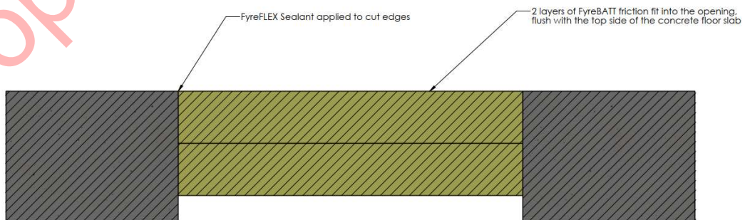
Figure 12 Blank seal protected with double layers of Trafalgar FyreBATT in floors— applied back-to-back
