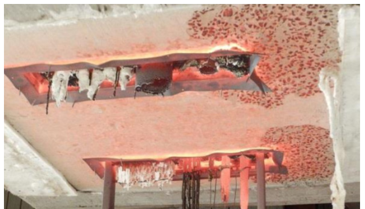
FyreBOX Cast-In after a 4 hour test.
