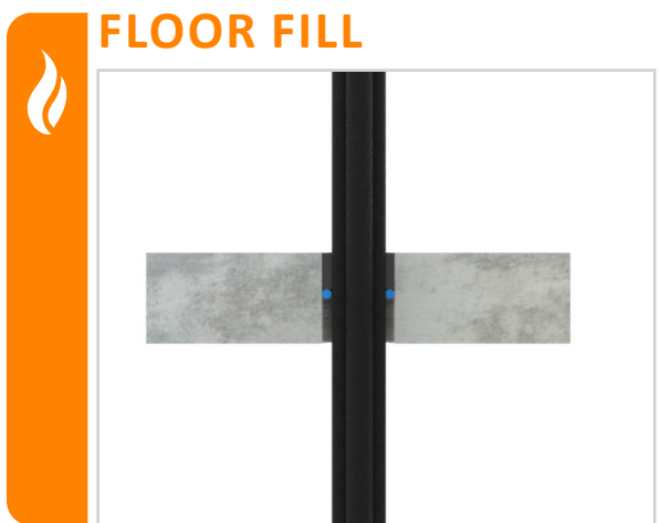
FyrePEX™ HP Sealant installed into Slab opening to a depth of at least 60mm from one side only. Refer to service specific requirements on page 11 .
