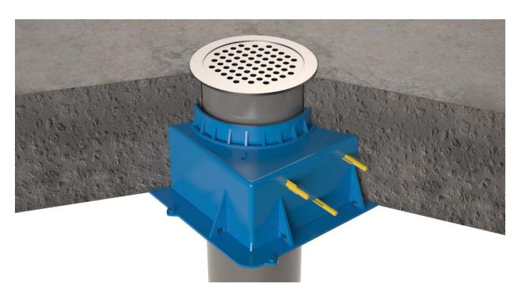
Floor waste collars help prevent the passage of fire and smoke through openings in compartment floors in the event of a fire. For installation of collars on permanent form work and in thin floor slabs (<150mm) please consult Promat. These collars are available in various models and their applications depend on the certification required for the building.
