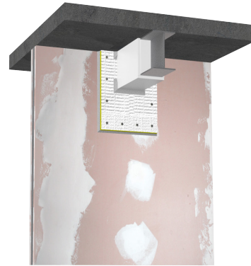
Batts (Surface Mounted/Friction Fitted) – Head of Wall with Corex
